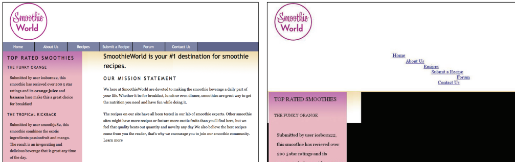
Your SmoothieWorld layout in a modern browser (left) versus Netscape Navigator 3 (right).
